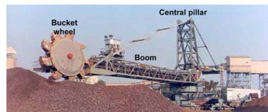
Fig. 1 Handling machine for material reclaiming
