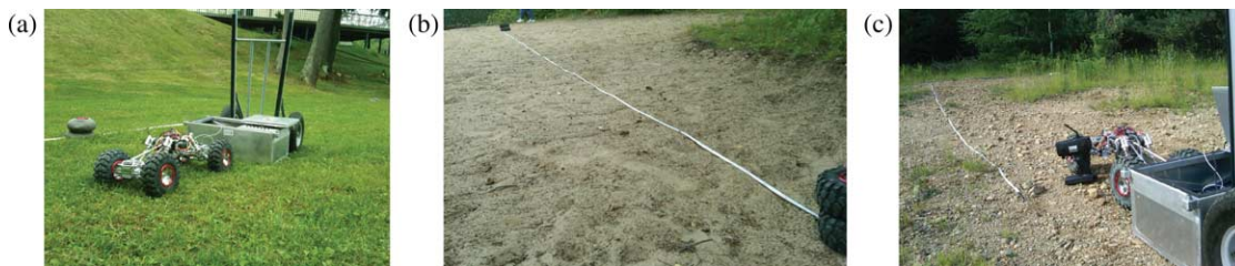
Figure 6. Terrain sites for vehicle testing. (a) Terrain 1: grass. (b) Terrain 2: soft sand. (c) Terrain 3: hard sand/gravel.
