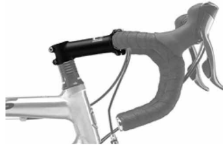
Figure 9. Stem is part of a bicycle that connects the handlebar to the fork.
