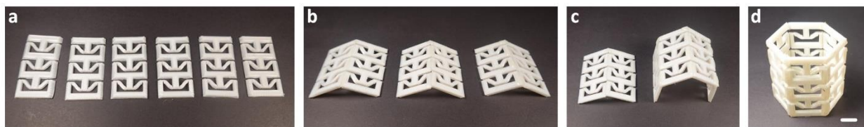
Figure S2. Manufacturing of hexagonal multistable guider. (a) 3D printed planar snapping strips. (b-d) Strip bonding to realize an extruded hexagonal cross-section. Scale bar = 1cm.
